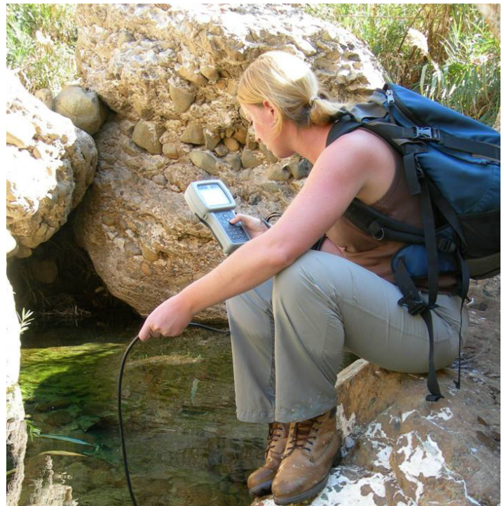
The YSI Model 556 being used in a wadi pool to measure several water quality parameters as part of the study.
